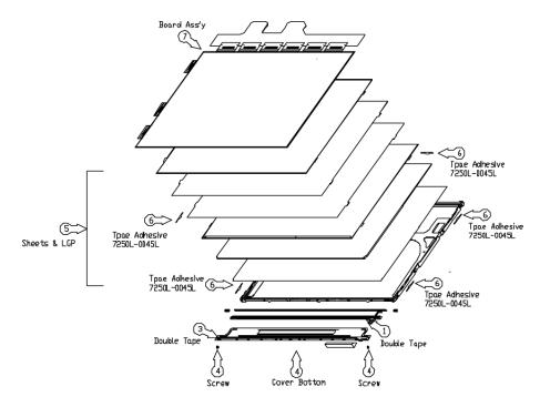
Figure 4-66 Replacing LG.Philips fluorescent lamp (WXGA) (5)
